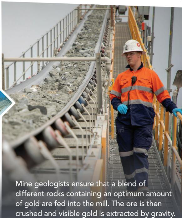
Mine geologists ensure that a blend of different rocks containing an optimum amount of gold are fed into the mill. The ore is then crushed and visible gold is extracted by gravity.
