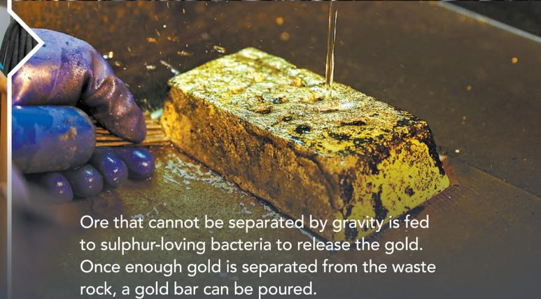
Ore that cannot be separated by gravity is fed to sulphur-loving bacteria to release the gold. Once enough gold is separated from the waste rock, a gold bar can be poured.
