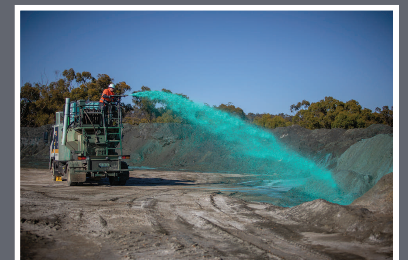
Applying chemical dust suppressants to tailings heaps.
